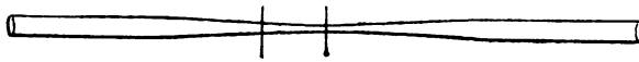
FIG. 40.—SHOWING WHERE TO CUT THE TUBE IN ORDER TO GET TWO DIPPING TUBES WITH DIFFERENT APERTURES
